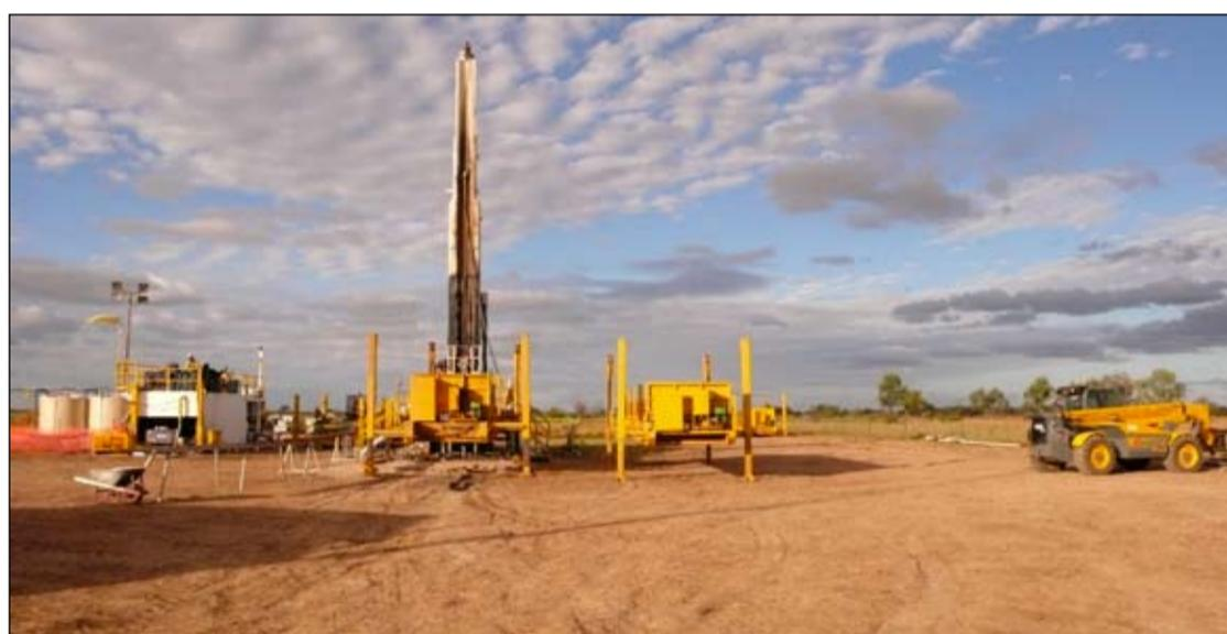
Exoma Energy drilling the Crossmore South 1 corehole on Crossmore Station in December 2009. Far left are two water tanks, then the mud tank and drill rig. On the right is a manatu (or four wheel drive fork lift). \* Photo courtesy Exoma Energy.
