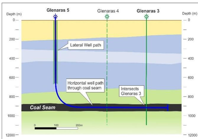
Modelling of a 350 m lateral in this R1 coal shows gas flows within three months. As a result, we now expect the pilot to be produced through to the end of the calendar year to see the full benefits of the lateral well. Final design work has now been completed. Timing for the project is weather dependent, but mobilisation to site is expected by mid-August 2016.
